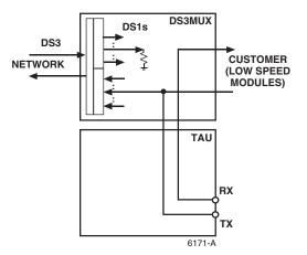
Figure 575-3h. Drop: Customer / Insert: Customer
